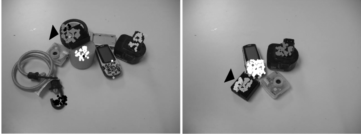
Figure 4: These are examples of errors from our program. The dots show where a feature was extracted by our saliency program. The shades of the dots indicate that a feature was categorized as the same type. The arrow on the left image shows an example of a merge. In this case a heat sink has been merged with a tire as a single object. In the right image the arrow shows a split where the heat sink has been split into two objects.
